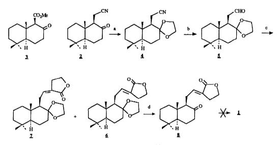
a) - Me<sub>3</sub>SiOCH<sub>2</sub>CH<sub>2</sub>OSiMe<sub>3</sub>, TMS- triflate, CH<sub>2</sub>Cl<sub>2</sub>, 0° C,<sup>10</sup>. b) - DIBAH, toluene, 0° C, 30 min., 80% yield. c) - diethylphosphono-2-butyrolactone, NaH, toluene, 0°C, then 5, toluene, 80°C, 1h, 80%, E/Z = 3/1. d) - HCl, 0.1 N, acetone.
